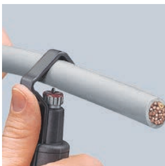
Setting the tool for circular cut
