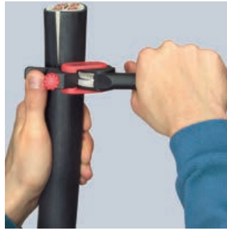
Turning the tool for circumferential cut
