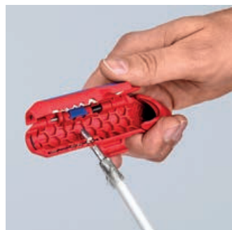
Stripping of a coax cable
