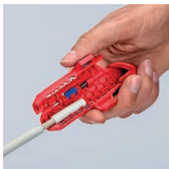
Stripping of a NYM cable
